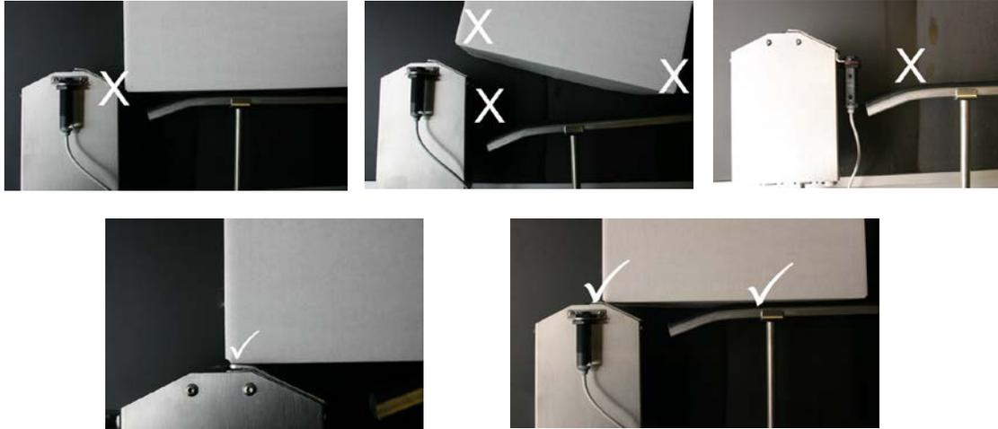
Decide on a position to mount the photocell product detector. The standard photocell is a diffuse reflective type (that is it 'sees' reflections from a product appearing in front of it). A retro-reflective type that uses a reflector as a mirror (that sees a product as an interruption between it and the reflector) is available from Codeology where diffuse reflective will not work.
