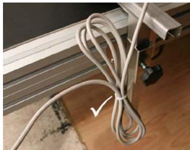
Do not hang cables over motors, or run alongside high voltage or motor drive cables or trunking. All of these may induce interference in the printer.
