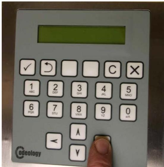
The control software is similar in operation to most mobile phone menu selections. A 'tick' key (✓) and a 'backup' key (◀) allow selection of an item on the screen, so scrolling until 'Dotsize' is shown on the screen then pressing ✓ takes the operator into the dotsize menu for example. Pressing ◀ takes the operator back out of the menu to where they started.
