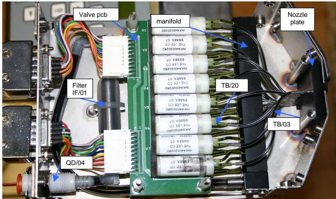
The valves are controlled from the control unit via a driver board and print head cable. The print sequence is triggered by a photocell detecting the box. The time waited between the photocell triggering and the print starting is called the print delay. The time that each valve is opened is called the dot size. How fast each dot follows the previous one is controlled by the speed.
