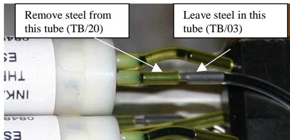
First remove the steel from the yellow TN/20 tubing where it leaves the valve. To do this, hold the TB/03 tube with a pair of long-nosed pliers and with your thumbnail ease the TB/20 from the steel. Take care when doing this for the first time as the tube is a tight fit.
