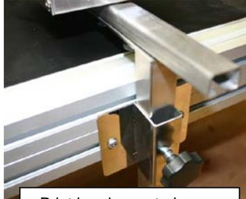
Print head mounted on an MF/01 bracket
