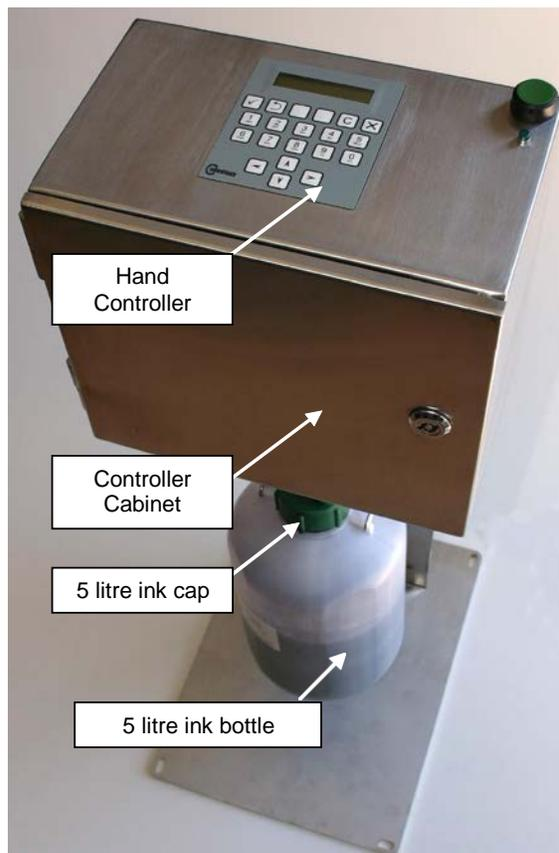
The controller cabinet houses the power supply (PSU), air pump, controller and hand controller. The air pump pressurises the ink bottle via the 5 litre ink cap. The ink is supplied from a 5 litre ink bottle that sits on an ink tray on the integral stand
